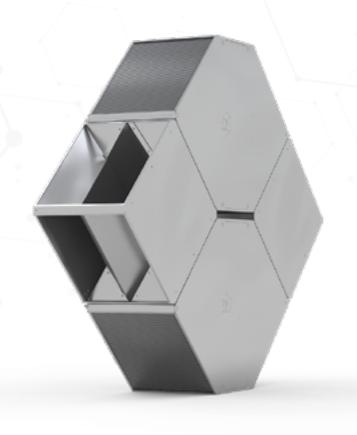
The COMBI solution is designed for recovery of **larger air volumes**. It consists of two REK+ or REC+ counterflow heat exchangers and two air dividers. The use of counterflow heat exchangers in the COMBI solution results in greater efficiency than with commonly used crossflow heat exchangers, which are also commonly employed for **higher flow** rates above 5,000 m³/h.
